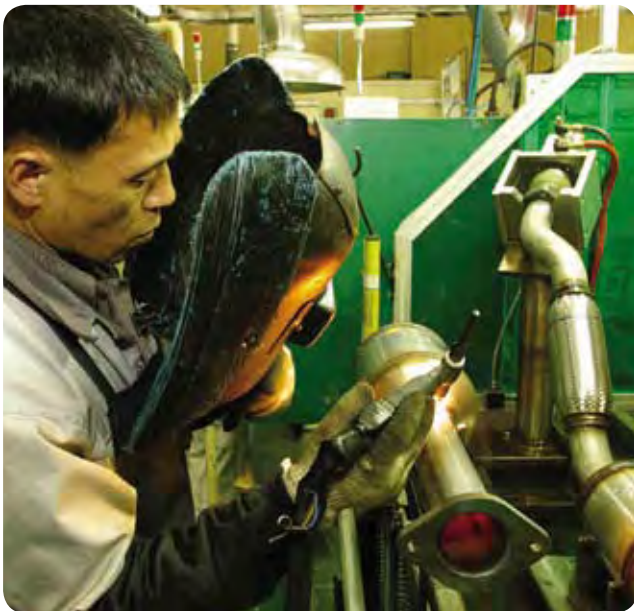
Exhaust system welding, grade 439, S. Korea.
