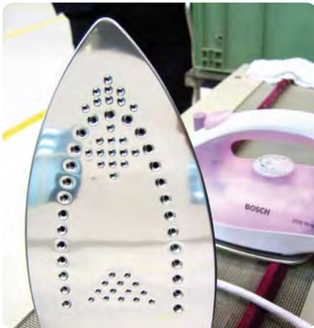
Soleplate of electric iron, in buffed grade 430.
