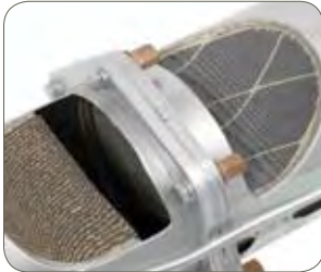
Grade 1.4509/441, diesel particle filter, Peugeot 607, Faurecia
