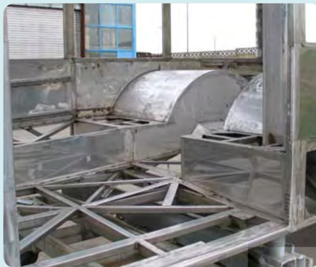
Welded structural frame in grade 1.4003.
